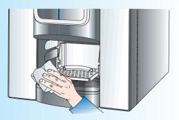
To avoid any risk of chemical oxydation or corrosion in general, use neutral detergents and avoid any solvent
