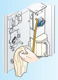
Clean inside the machine with a neutral detergent solution by using a piece of cloth that is slightly wet.
